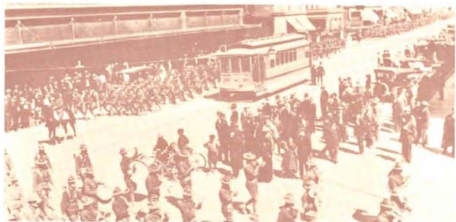
Fig. 12: Car number 90 running down G Avenue in about 1917 or 1918 shares the right of way with a parade. Originally from San Diego, the California style car has skirting or steps running the full car length and is moving away from the camera in this picture. (Photo from Gene Caywood Collection)
